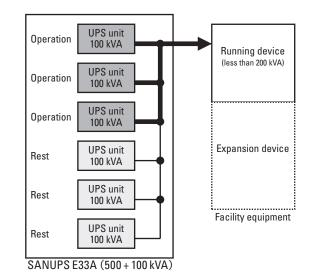
Fig. 4: Settings for resting device in a 500 + 100 kVA system implementation
